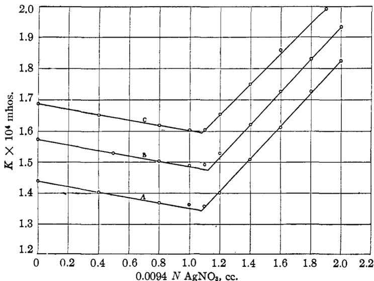
For curve B subtract 0.1 from value of  $K$ ; for curve C, subtract 0.2.
